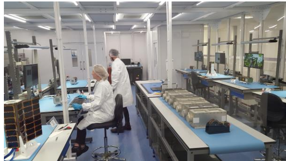
Figure 3-4 Spire technicians assemble a batch of Lemur satellites. 9
